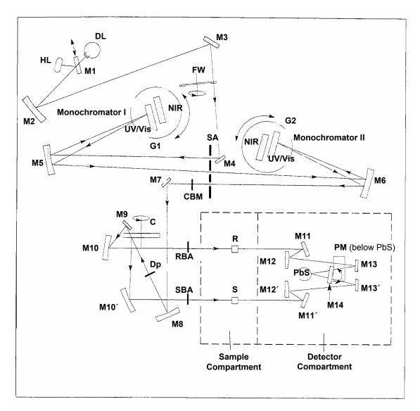
Figure 7 Schematic of Optical System
