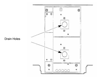
Figure 17 Drain holes in standard sample compartment baseplate
