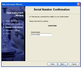
9. Check the serial number on the right-hand side of the instrument, where the PC connects to the instrument, correct it if necessary, and click **Next**.
