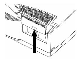
Figure 20 Removing the lamp cover
