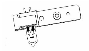
**Figure 19 Pre-aligned Halogen Lamp**
