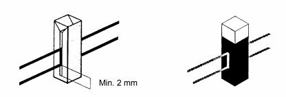
Figure 15 Correct alignment of the radiation beam in the cell sample area
