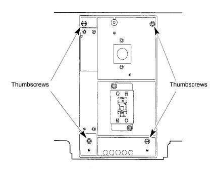
Figure 24 Four thumbscrews on the sample compartment baseplate
