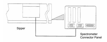
Figure 30 Sipper, electrical connection
