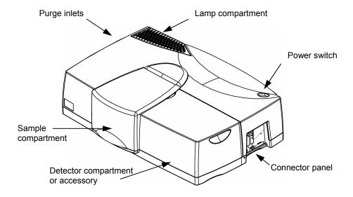
Figure 6 Lambda 650/850/950 spectrometer features
