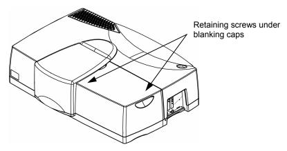
Figure 26 Undoing the retaining screws
