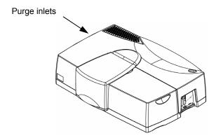
Figure 16 Connectors for the purge gas supply
