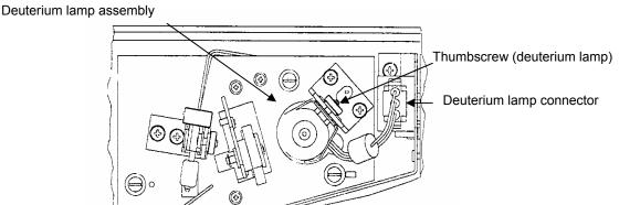
Figure 23 Removing the deuterium lamp connector
