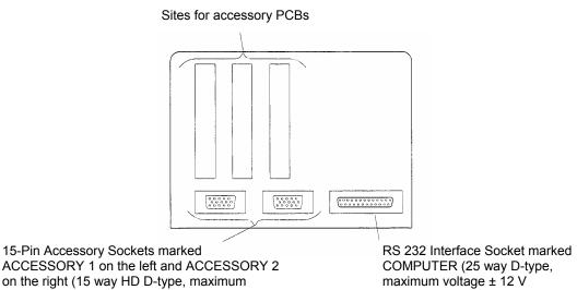
**Figure 28 Connector Panel for Accessories**
