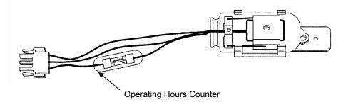
Figure 22 Pre-aligned Deuterium Lamp Assembly (B0160917)
