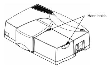
Figure 27 Removing the detector compartment cover
