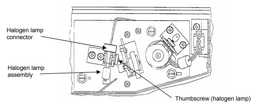
Figure 21 Removing the halogen lamp connector
