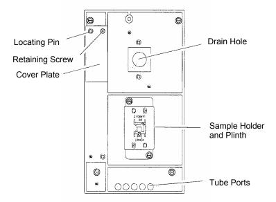
Figure 14 Lambda 650/850/950 Sample Compartment Baseplate
